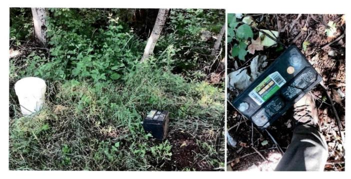
**Photo 7 and 8:** Leaky gasoline-powered generator lacking containment adjacent to Paynes Creek. Use, refueling, and placement of this generator places petroleum products where they can enter waters of the state.
